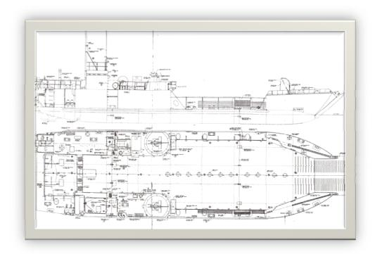
Clearer deck plan drawing of the LCT Mark 6. The engine hatch Tom had to use is shown just under the catwalk that ran between the compartments. The holes shown in the deck were for tying down vehicles. The space below the holes in the deck came into play during the "Applejack incident."
