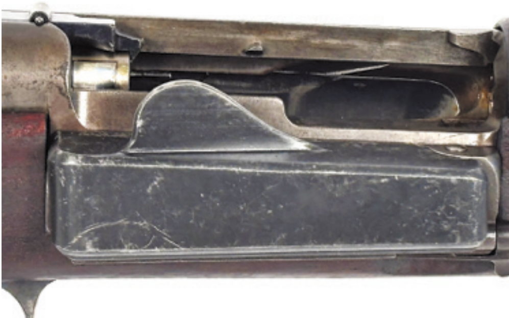
Figure 15: Photo of the open breech-note the small pin on the left side of the receiver
