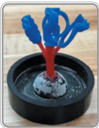
A completed sprue tree. After weighing, it will be ready for investing.
